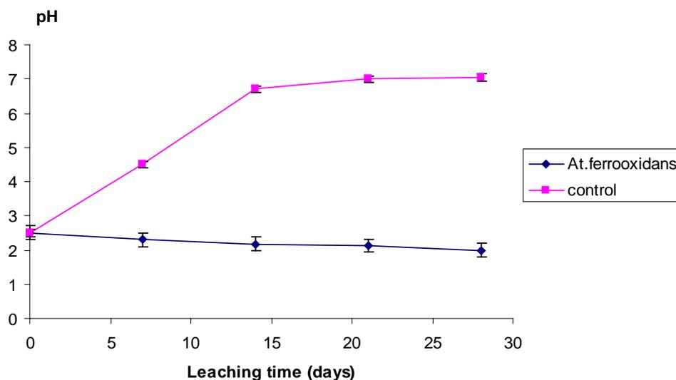
Figure 1 - pH profiles of leach suspensions during experiments
