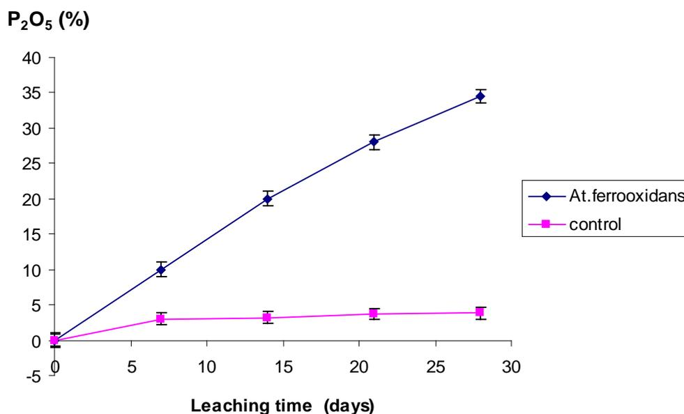
Figure 2 - Percentage phosphorus recovery (% P<sub>2</sub>O<sub>5</sub>) from phosphate ore during leaching experiments
