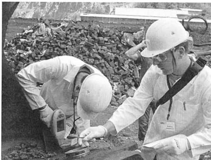
Fig. 3: Field determination of heavy metal content with NITON X-ray fluorescence analyzer.
