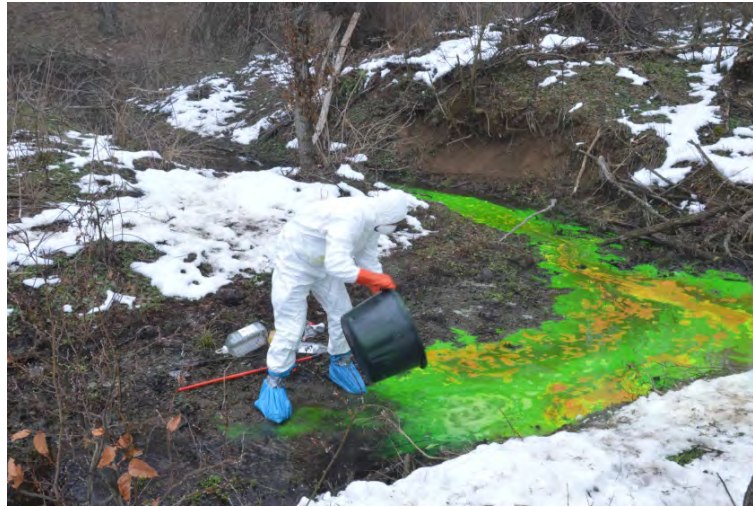
Fig. 3 Dye test – verified connection of the Cvetanovac ponor and Blederiya mixed spring
