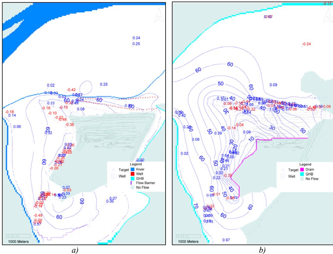
Picture 5. Positions of piezometrical levels in a) - gravelly b) - sandy layer above the third (III) coal seam at the end of the period for which is carried out recalibration model (December 2015)
