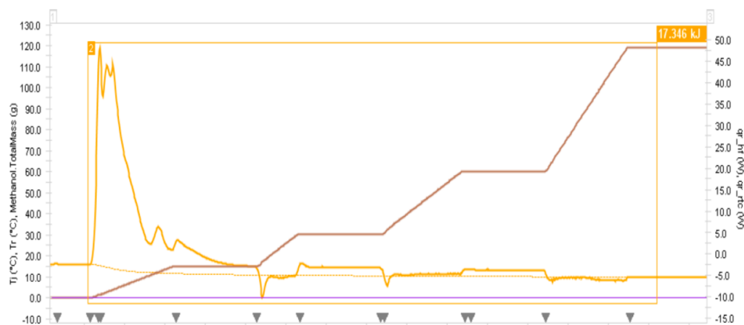
Figure 5. Heat evolution during addition of methanol to the borane reduction mixture.
